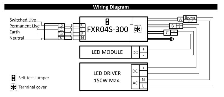
The terminal cover provides access for battery disconnection and replacement and is secured in place with a single screw from the back of the unit, remove this screw to gain access.
