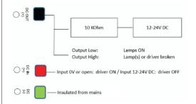
Power Input: 3 pin connector to connect with min 18AWG
